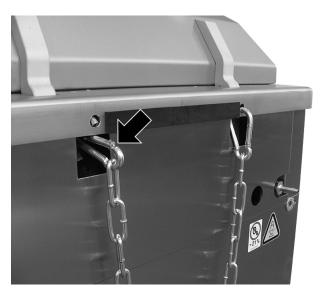
Undo the chain on one side on the rear of the machine.
