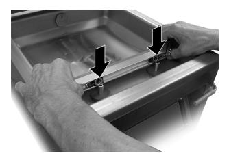
> Install the sealing bar in such a way that the screws on the sealing bar point to the middle of the chamber.
