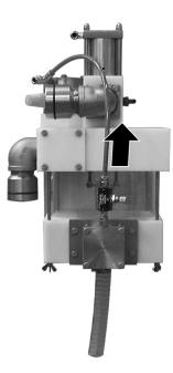
> Release the winged nuts and the retaining rings on the base of the liquid separator.
