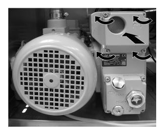
> Fasten the safety guard on the back of the machine.
